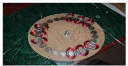
Fig.6 Magnet placing on stator
