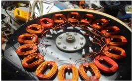
Fig.2 stator and coils arrangements
